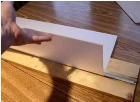
2) Fold wing completely in half, lay flat object to hold folded wing flat and use razor knife to trim both sides of the fold exactly the same length (very important) (Trimming the TE is shown below)
