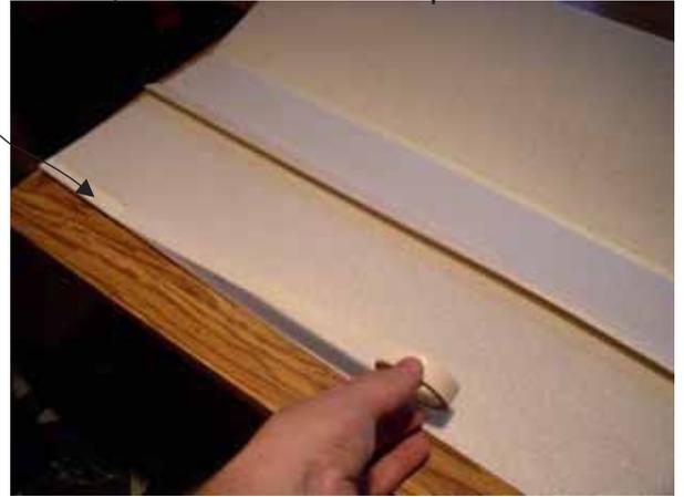
3) Use tape to secure bottom edge of spar to inside of wing, laying forward, so that it can be rotated up and against the servo after folding the wing and securing the trailing edge. Fold wing flat first.
